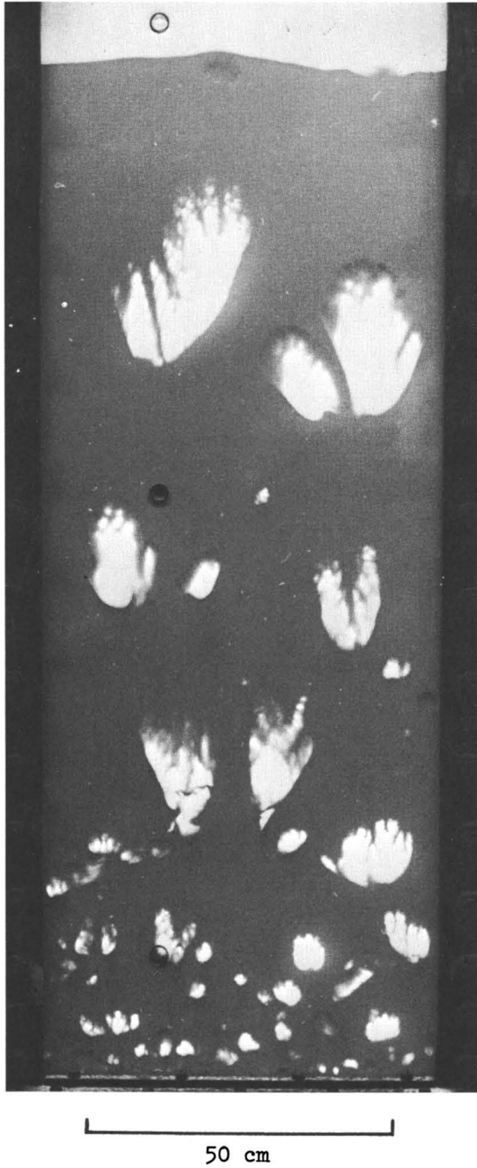
Figure 1. Bubbles in a two-dimensional fluidized bed.
